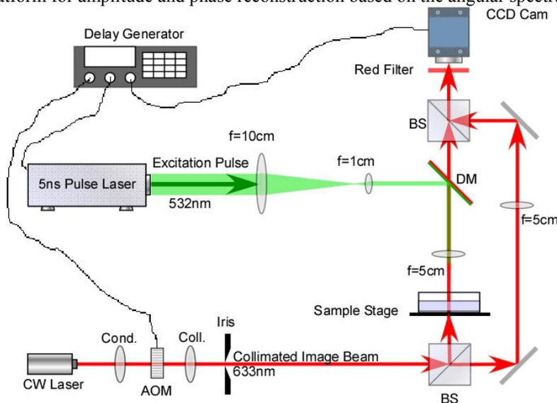
Fig. 1. Experimental apparatus. Pulsed excitation beam (green); Imaging beams (red); Microscope Objective (MO); Beam Splitter (BS); Dichroic Mirror (DM); Acousto-optic Modulator (AOM).
