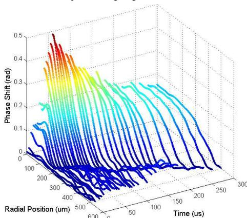
Fig. 2. Phase profile response as a function of radial distance from the center of the structure at each time interval.
