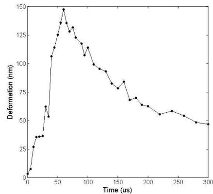
Fig. 3. Physical deformation height of the center of the structure as a function of time.
